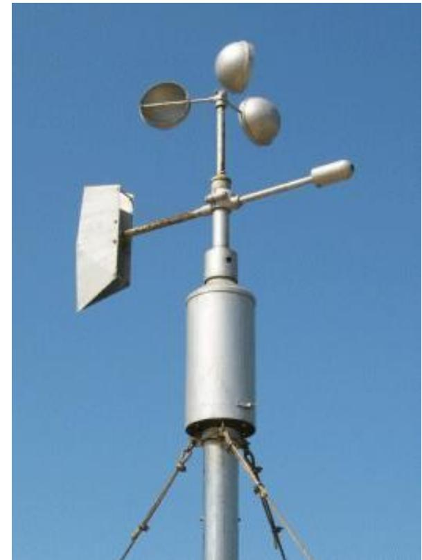
**Wind Vane:** A weather instrument used to determine the direction the wind is blowing.
